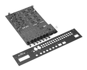
To upgrade a transmitter without an optical network connection (LBB 4502 range) to a transmitter with an optical network connection (INT-TX range) a Transmitter Upgrade Kit (INT-TXK) is required. The upgrade kit comprises the main PCB of the transmitter, a rear panel, a glue stud and a screw for mounting the main PCB in the housing of the LBB 4502 transmitter.
